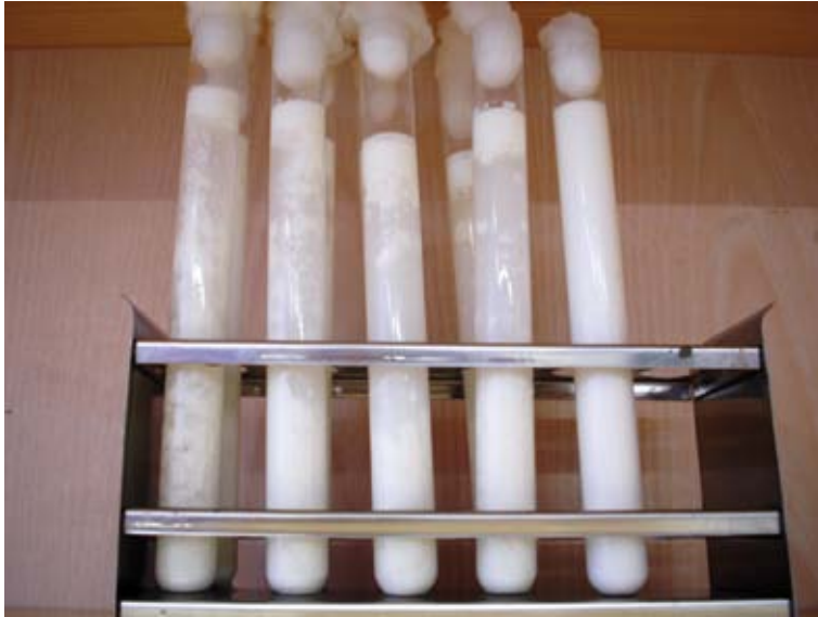
Fermentation assays with milk fermenter to detect Coli aerogenes
