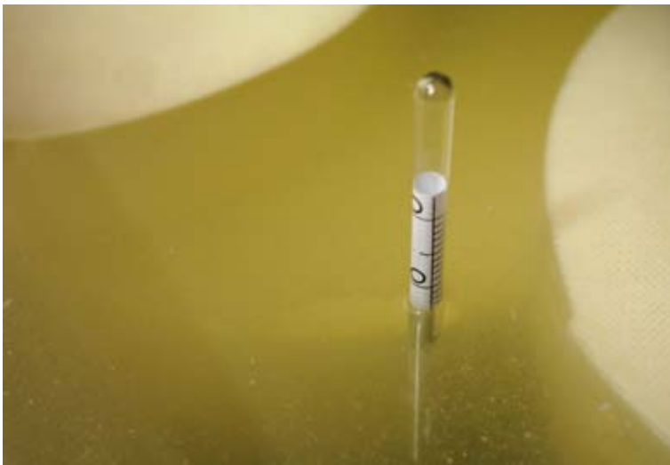
Salt concentration control in brine bath
